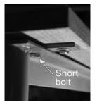
Remove the two short bolts and reposition in seat bar for slight adjustments. Remove short bolts and rotate seat 180 degrees for a large adjustment. Always tighten carefully to aviod injury.
